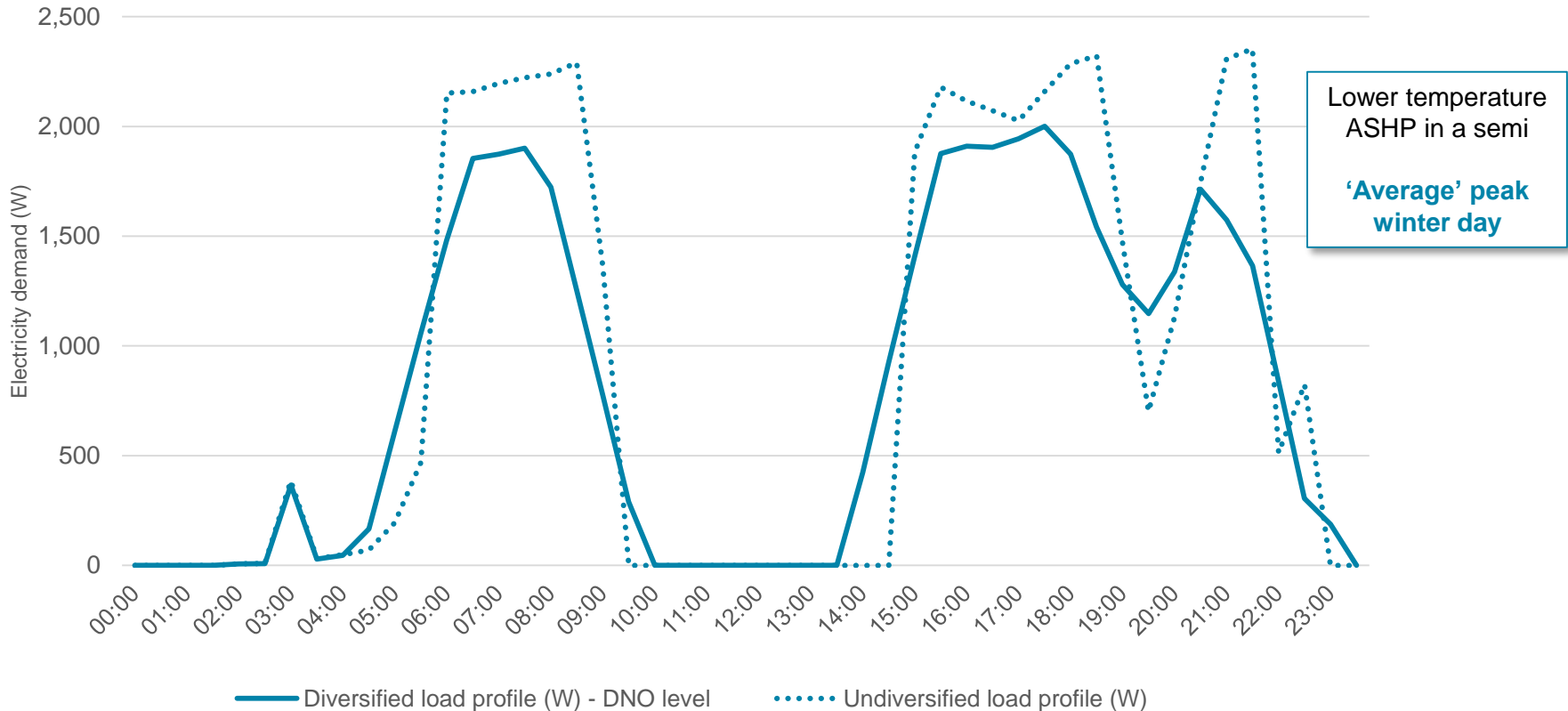
Undiversified vs diversified (@ DNO level) load profiles for a LT ASHP in a semi on an 'average' peak winter day
