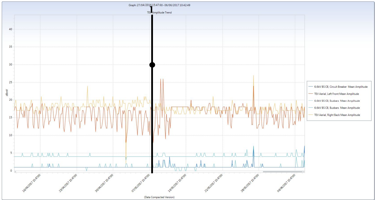
Figure 12 TEV Activity Plot with Date of Fault overlay for All TEV Channels Covering Fault in Littleborough
