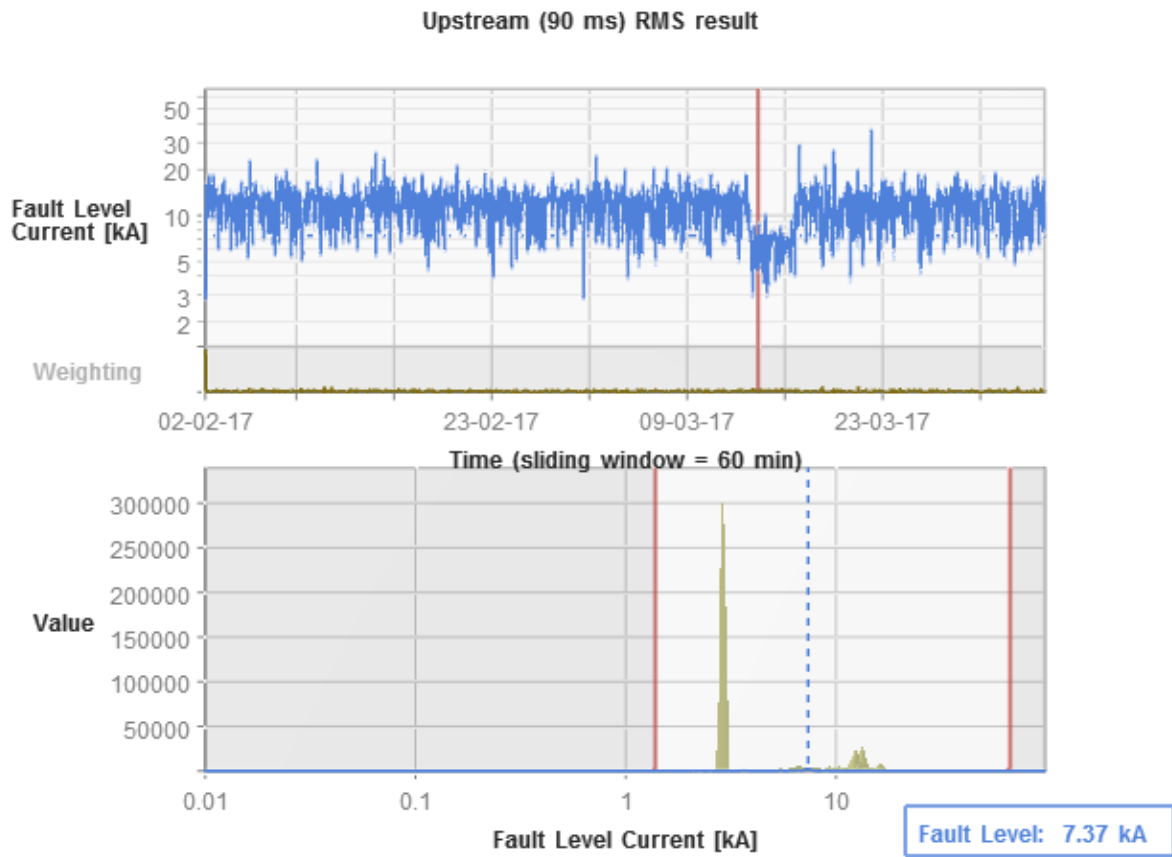
Graph 42. Second half recording. RMS Break Fault level at 90ms, 2% filtering.
