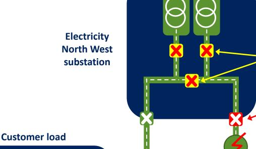
Adaptive Protection is only enabled when fault level is exceeded then either the transformer breaker or bus section breaker operates before the feeder breaker reducing fault current
