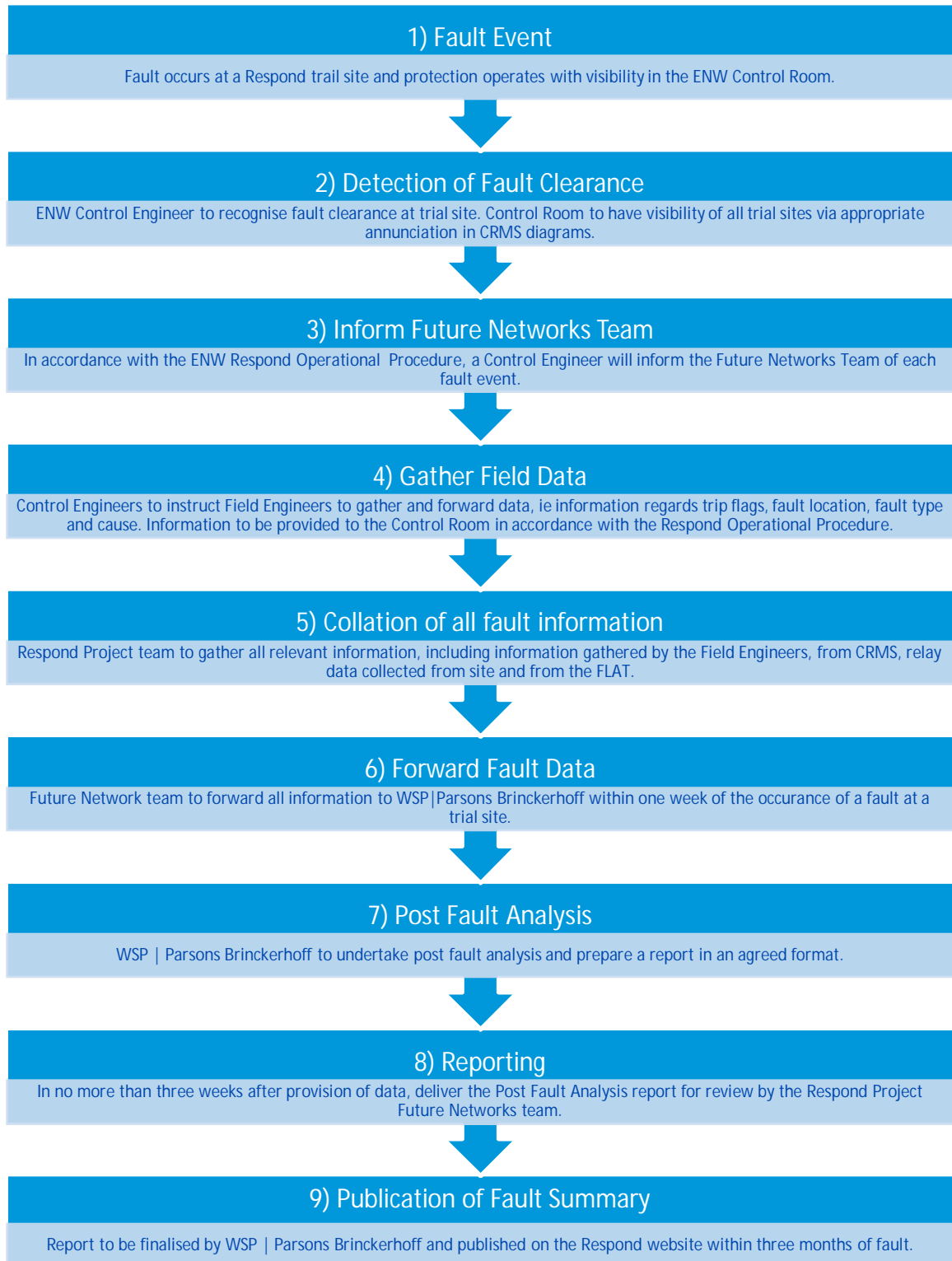
Figure 0-1: Post Fault Analysis Process
