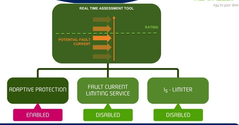
The technique will only operate when the fault level is exceeded and FLAT enables the technique, then we need to have a network fault.
