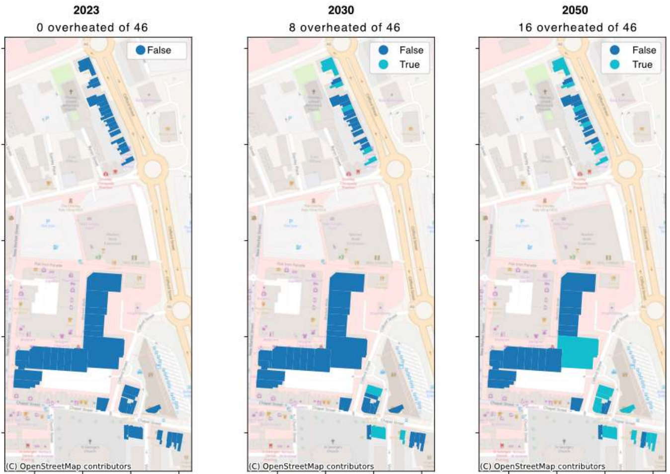
Figure 3: Simulated overheating for the years 2023, 2030 and 2050 in the Cattle Market dataset given constant 2023 levels of cooling
