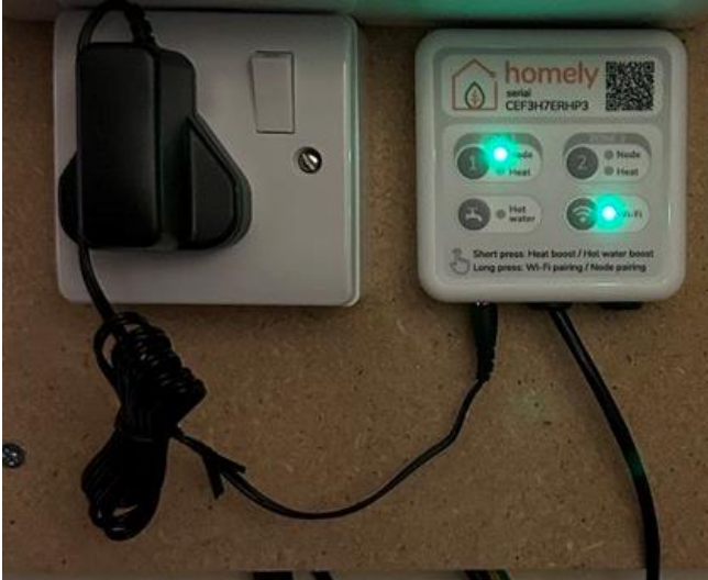
Figure 2—3 Supplier 1 HEMS manual user override
