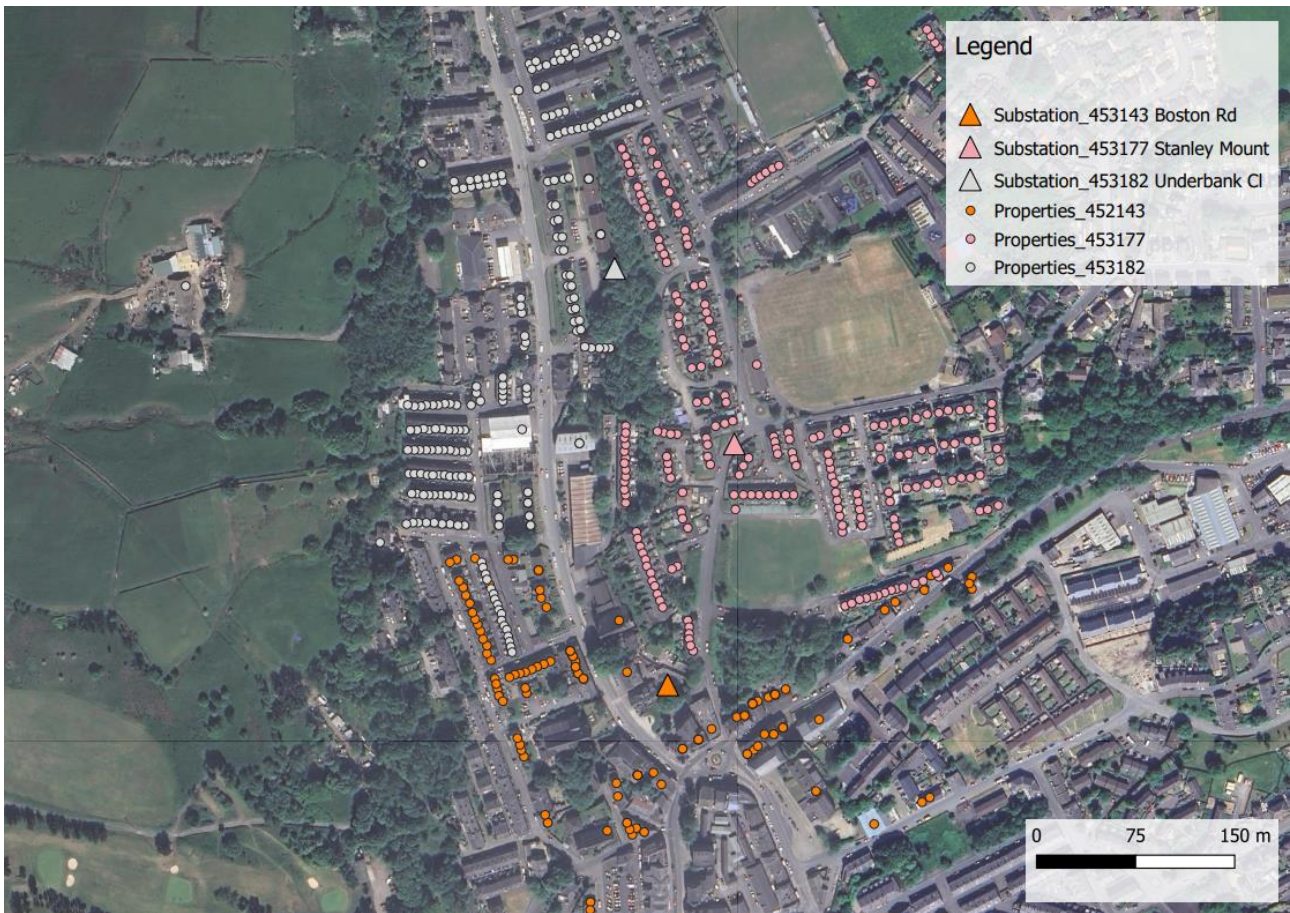
Figure 3-2 Properties mapped to secondary substations
