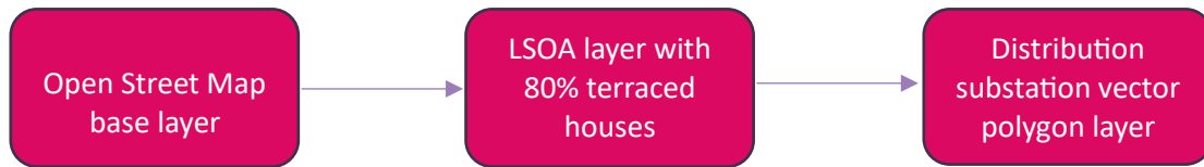
Figure 3-1: Information layers on GIS map for identification on potential NZT SLES locations
